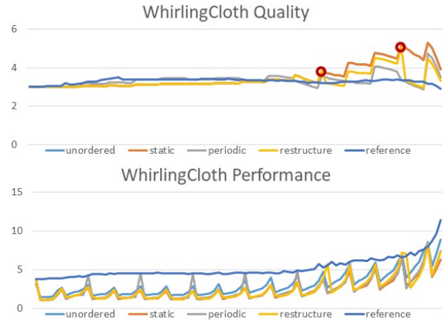
Figure 8: Five curves of five strategies for Whirling Cloth benchmark tested on GTX1080. The red circles indicate a BVH restructuring event. Since the number of related front nodes are above the threshold, the BVTT fronts at both events are reconstructed right before further degenerations. The time interval between these two events is small, so the benefits are unfortunately soon offset by their overhead.
