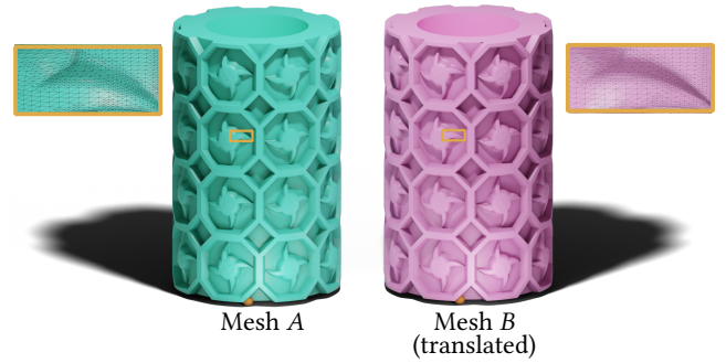
Fig. 2. Mesh A has 2.274 M faces and mesh B has 1.137 M. Our method terminates with a certified interval satisfying the stopping tolerance \epsilon = 10^{-6} for this near-zero Hausdorff distance case. The points on the bottom are the maximizer on A and its closest point on B ; the close-up views illustrate the high resolution of both meshes.
