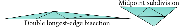
Fig. 4. Very thin triangles are subdivided using a double longest-edge bisection while better-shaped ones are subdivided using midpoint subdivision.
