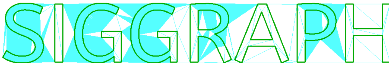
Fig. 1. Letters benchmark. For a scene containing approximately 900K vertices with numerous constraints of varying sizes, g CDT achieves an overall speedup of roughly 25X over the prior state-of-the-art GPU-based CDT algorithm gDel2D [Qi et al. 2013, 2019], while the constraint-processing component is nearly three orders of magnitude faster.
