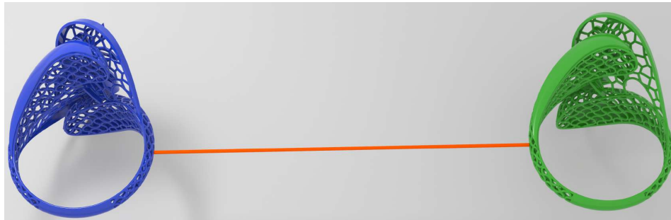
Fig. 1. Benchmark Rings: For the pair of rings, each consisting of 7.5M triangles, our algorithm can calculate the minimum distance between them (as indicated by the orange line) within 0.38 milliseconds on an NVIDIA GeForce 4090. As compared to an optimized CPU implementation (PQP [Larsen et al. 2014]), we observe 54X speedups for this specific frame and an average speedup of up to 26X across a sequence of rotation frames.
